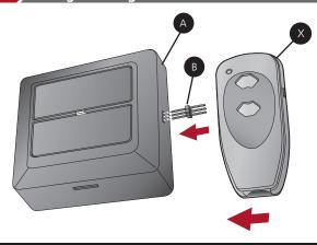
Connect transmitter (X) and wall control station (A) by using the programming connector (B).
