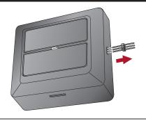
Disconnect transmitter and remove programming connector.
