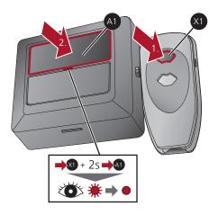
Press and hold the designated transmitter button (X1). The hand-held transmitter LED lights up. Then press and hold the desired button (A1) on your wireless wall control station (A). The transmitter LED flashes and lights up steady after 2 seconds. Release both buttons – programming is complete.
