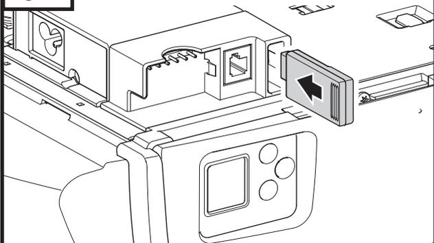
**Fig. 35** Terminal block XB03
