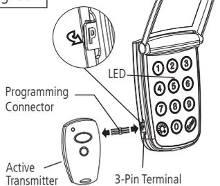
**Make sure the programming connector is inserted all the way into the programming port.**
