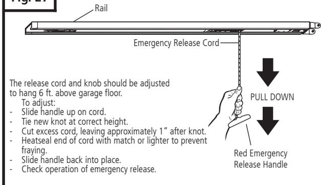
The emergency release cord with red handle which is already attached to the trolley, are extremely important parts of the operator system Fig. 27. Pulling the release cord disengages the door from the opener. This allows the door to be moved manually up and down independent of the opener motor.
