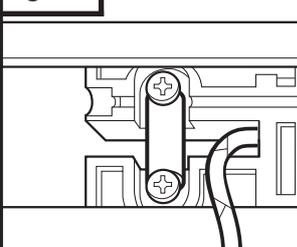
Fig. 18B Incorrectly seated pin.
