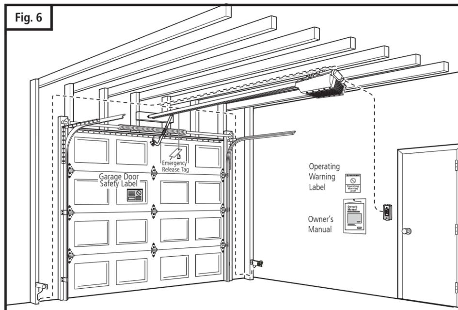
Shown on the right is an overall view of a completed garage door operator system installed on a sectional door. The arrangement is similar for a one-piece door (except for differences described later in this manual).
